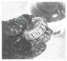
Work fresh wheel bearing grease through the cage and the inner race. There are tools you can buy to make packing quicker and cleaner, but the manual method works perfectly well.
