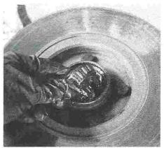
On the Spitfire, there's a felt dust seal and an inner cap that must be removed to get at the inner wheel bearing. The dust seal will need to be replaced.
