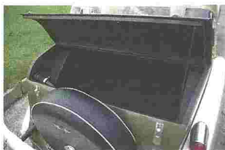
Where most Plus 4s have a sloped deck, the prototype features a weather-tight trunk big enough to hold a golf bag. Hydraulic mounts help the bumpers meet the federal 5-MPH impact requirement.
