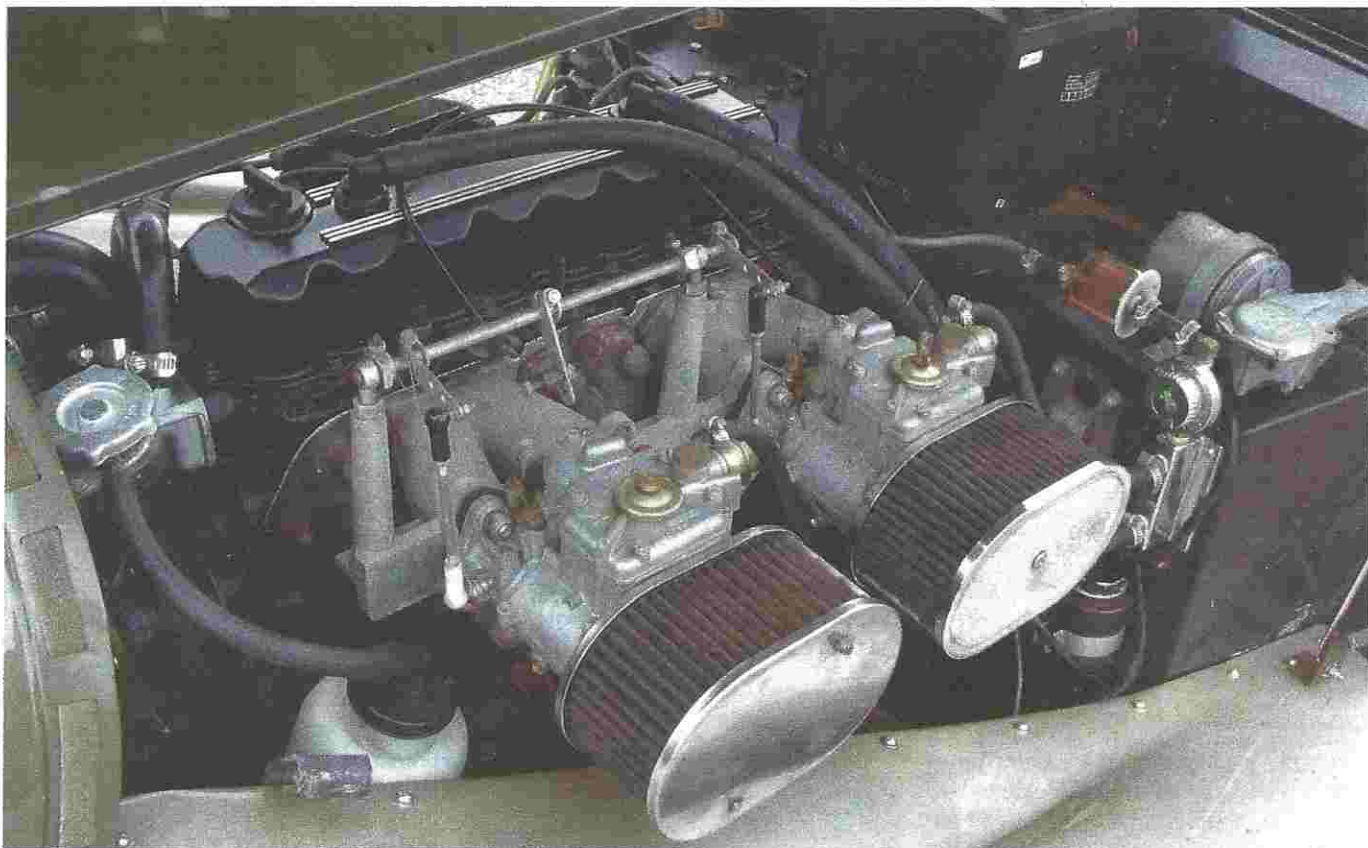
The AMC 2.5-liter four was an EPA-certified engine that Morgan could have used to reintroduce the Plus 4 to America. Equipped with twin sidedraft Webers in place of fuel injection, the pushrod four fits in the space once occupied by a Triumph TR4 engine, and makes an estimated 150-170hp.
