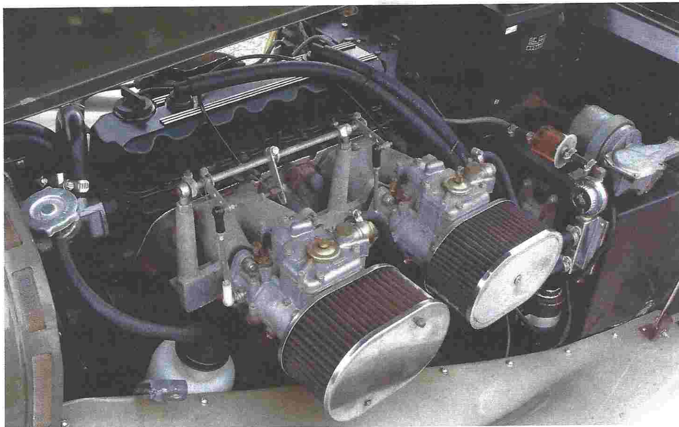
The AMC 2.5-liter four was an EPA-certified engine that Morgan could have used to reintroduce the Plus 4 to America. Equipped with twin sidedraft Webers in place of fuel injection, the pushrod four fits in the space once occupied by a Triumph TR4 engine, and makes an estimated 150-170hp.
