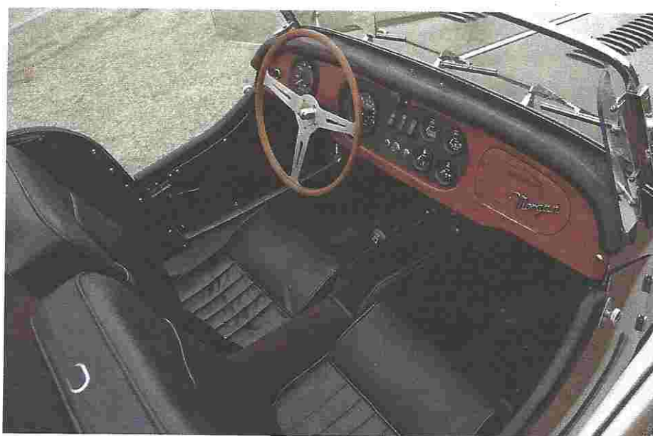
The comfortable leather seats are from a Morgan Plus 8, with their headrests removed. The tunnel had to be enlarged to house the five-speed's bell housing, cutting into the available footroom.
