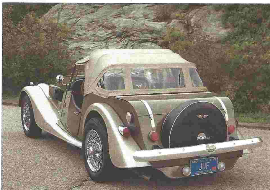
Where most Plus 4s have a sloped deck, the prototype features a weather-tight trunk big enough to hold a golf bag. Hydraulic mounts help the bumpers meet the federal 5-MPH impact requirement.
