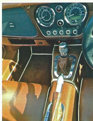
A central speedo and tach—with start button below—and turned metal for gear lever and hand-brake contrast with downmarket plastic airbag paneling.
