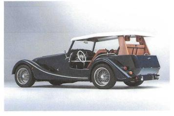
There are no doors, for a start, and the rear bodywork has been cut back as low as possible. Shade is provided by an aluminum canopy, which swings upwards on both sides to allow up to four passengers easy access to the wonderful interior, finished in tan hide and white basketweave.
