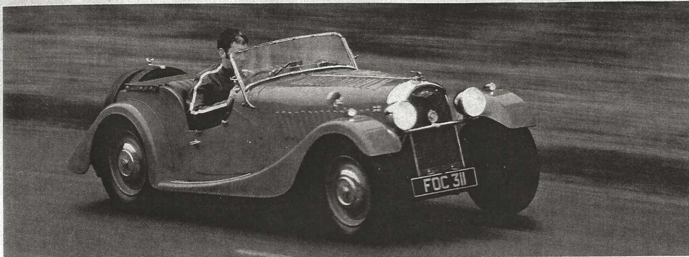
Torquey Morgan 4-4 added a fourth wheel and established the Morgan look and structure – steel chassis bearing an ash frame covered with metal panels
